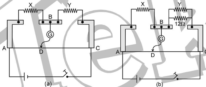
**F.8** The meter-bridge wire AB shown in figure is 50 cm long. When AD = 30 cm, no deflection occurs in the galvanometer. Find R.
