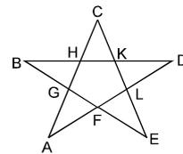
**B.15** The resistance of each resistor in the circuit diagram shown in figure is the same and equal to  $R$ . The voltage across the terminals is  $U$ . Determine the current  $I$  in the leads if their resistance can be neglected.
